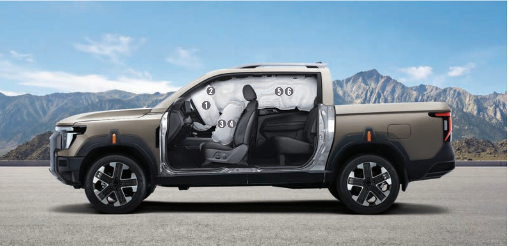
6 airbags 1. Driver airbag 2. Passenger airbag 3/4. Driver & passenger side airbags 5/6. Curtain airbags
