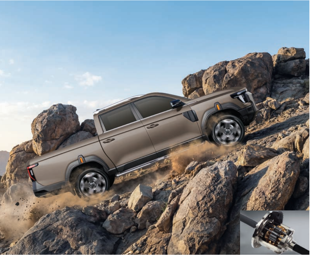
Locking Differential On mud, snow or other slippery surfaces, one wheel may slip or lift into the air. In such circumstances, the locking differential locks both wheels on the same axle together so they turn in unison, allowing the vehicle to recover its traction and momentum.
