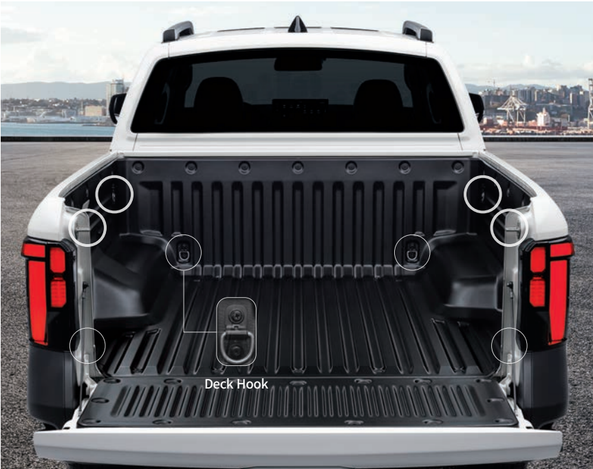
Deck Hook Increased from four to eight hooks to secure various loads more firmly and enhance cargo stability.
